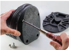
Insert 4 self-tapping screws
